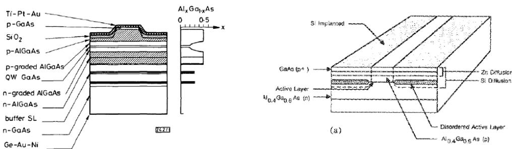
Figure 2: Cross section of a ridge waveguide [34] and a silicon implanted impurity disordered waveguide [31] laser diode on GaAs substrate
