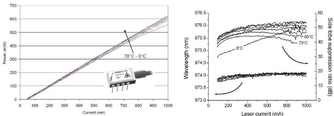
Figure 1: Performance of an uncooled 980nm MiniDIL for undersea systems (courtesy Bookham)
