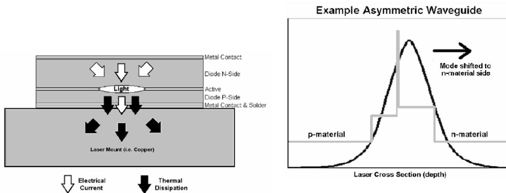
Figure 5: Cross section of “junction-down” mounted BA diode laser and example of asymmetric LOC waveguide [21]
