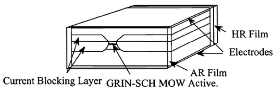
Figure 8: Schematic structure of a 14xxnm diode laser chip [135]
