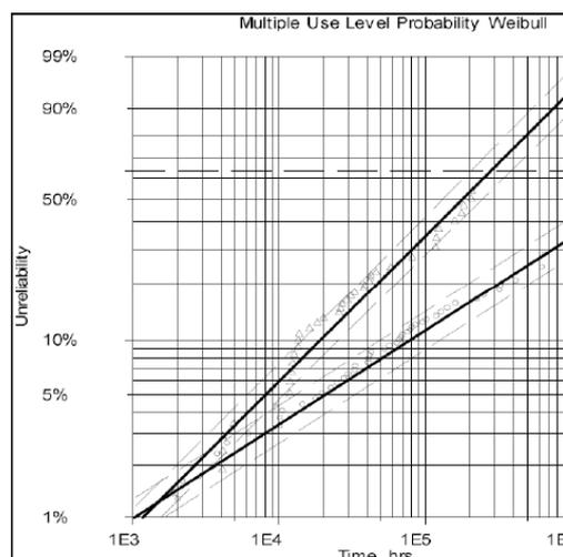
Figure 12: Projected percentage of failures as function of time, based on multicell test, for use conditions of 8W, 30<sup>0</sup>C for two types of 100µm BA diode lasers. Projected time to 5% failures are for the two types of BA diode lasers 8'000h and 20'000h, respectively [156]
