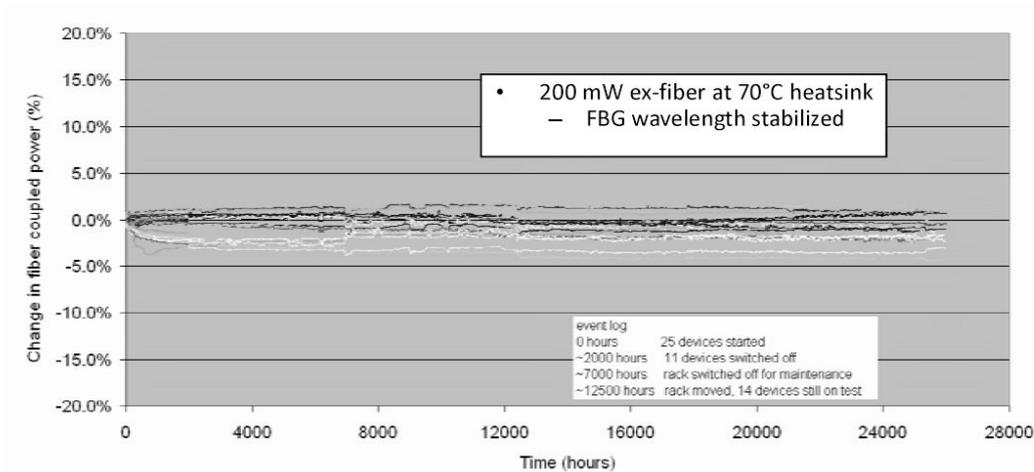
Figure 6: Stability of 25 uncooled FBG stabilized 980nm pump diode MiniDIL over 3 years of high temperature and maximum power operation, courtesy Bookham
