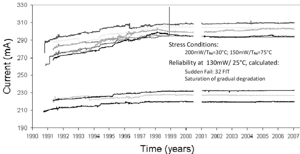
Figure 7: 16 years of constant power operation of 980nm pump diodes at temperature and power stress, courtesy Bookham
