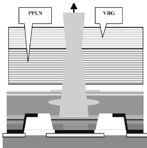
Figure 13: Schematic structure of a NECL array element of a visible light source by frequency doubling [176]
