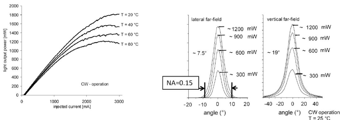
Figure 4: Light output versus injected current of ridge waveguide laser at various heatsink temperatures and farfields at various power levels [56]
