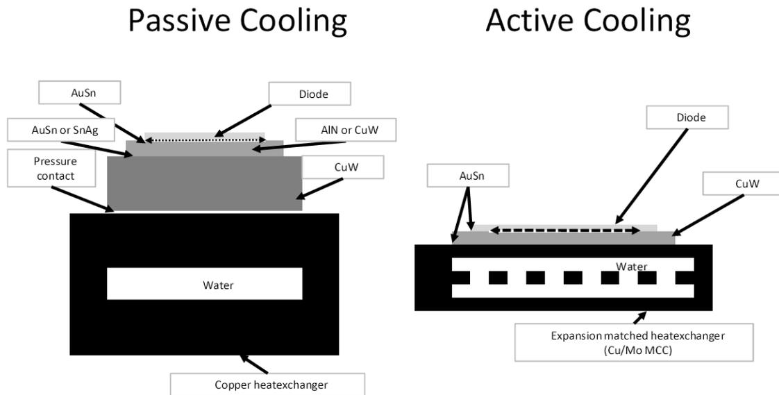
Figure 9: Schematic structure of a passive cooled diode laser and an active cooled diode laser
