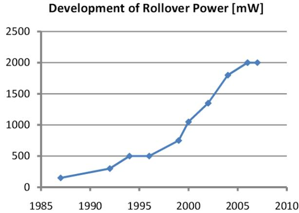
Figure 3: Development of roll-over power of 980nm single lateral mode pump diodes (cw, junction up, at room temperature)
