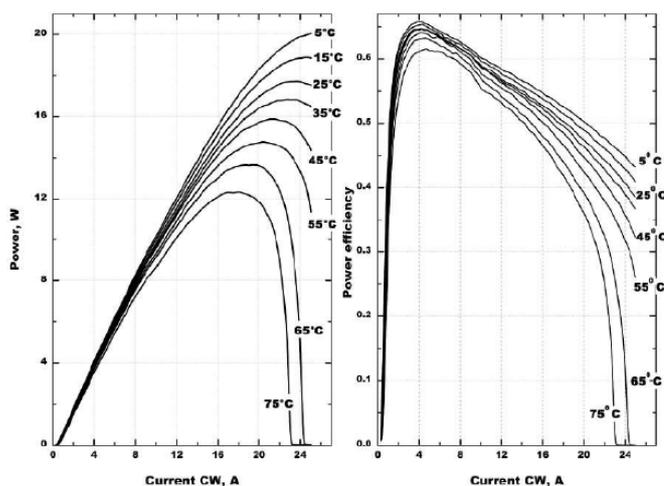
Figure 11: Typical roll-over characteristics and power conversion efficiency as function of current (at various heatsink temperatures) for a 90 $\mu$ m wide BA diode laser [155]
