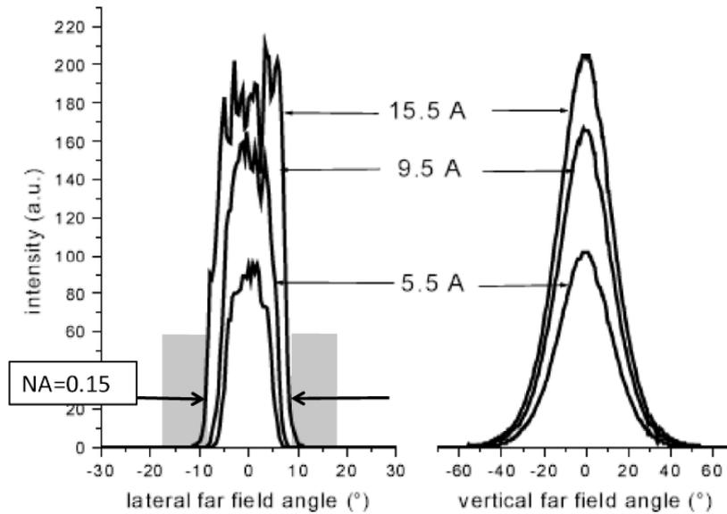
Figure 10: Slow (lateral) and fast (vertical) axis farfields of a 90 $\mu\text{m}$  BA diode for various drive currents [147]
